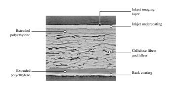
Figure 1. Cross section of an inkjet photographic paper
